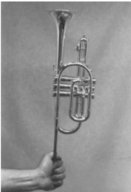
Cornets and trumpets should be held by the receiver. An old mouthpiece soldered to a brass rod makes a good holder.
