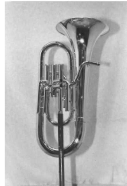
A one inch pipe attached to a flange located in the lacquer booth floor serves as a rigid base for the wooden holder. The pipe is easily removed when not in use.
