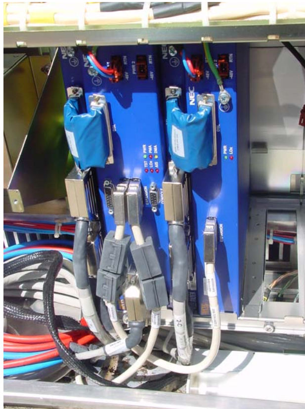
AM35 Mounting frame and Modules positioned into a 2G480 RIM Housing.
