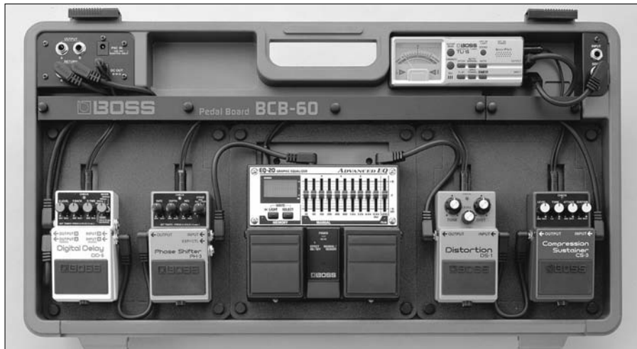
Figure 15-18: The stomp box solution.
