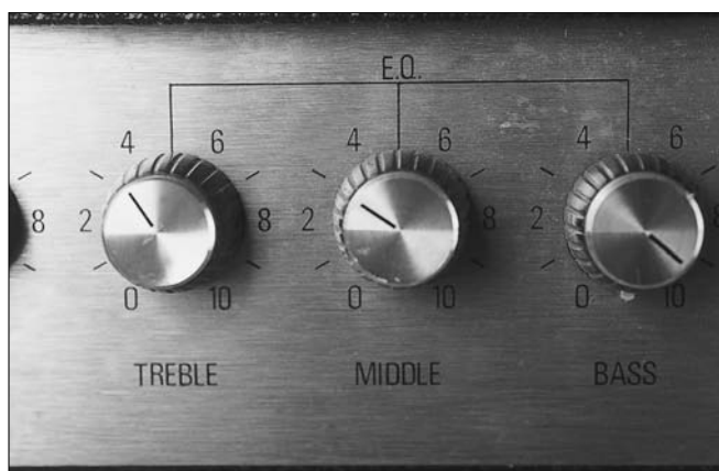
Figure 15-6: The tone section of an amp.
