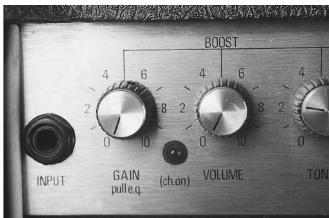
Figure 15-5: The preamp section of an amp.
